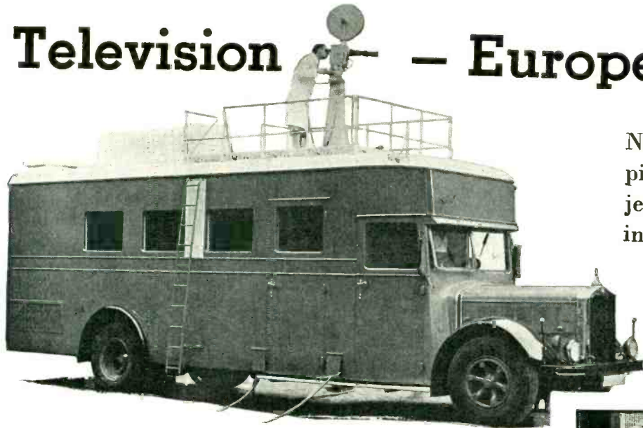
This truck, the second of its kind constructed in Germany, is fitted to develop the film taken by the camera on its roof, and scans the film immediately for transmission. The whole process of development and scanning consumes thirty seconds
