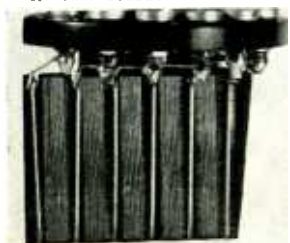
Aryton-Perry windings of the 1-, 10-, and 100-ohm decades. The 1,000- and 10,000-ohm decades are unifilar windings on mica cards.
