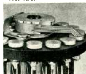
Quadruple-leaf, phosphor-bronze switches. Contact surfaces of leaves are ground flat to act as four independent brushes. Contact resistance only 0.002 ohm.
