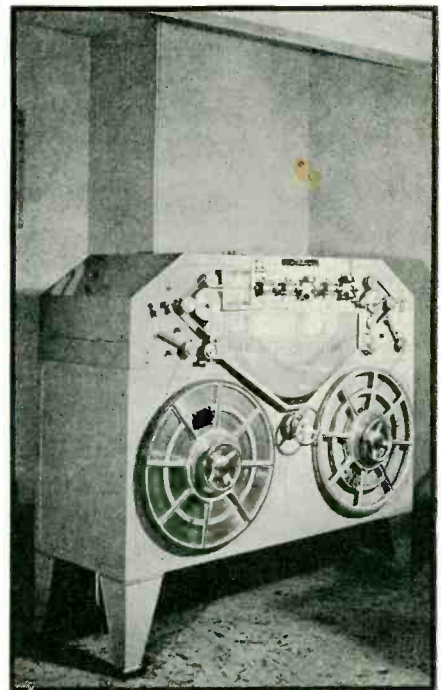
A large percentage of the programs sent over the British short-wave system are magnetic recordings made from previous broadcasts. Above is one of the Blatterphone units used by the BBC
