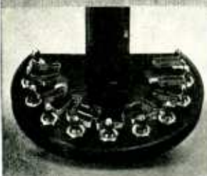
Bifilar Manganin winding of 0.1 ohm decade
