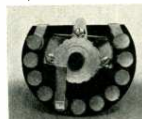
Contact studs \frac{3}{8} inch in diameter, ground flat. Cam-type positive detent mechanism. Entire unit shielded behind panel.
